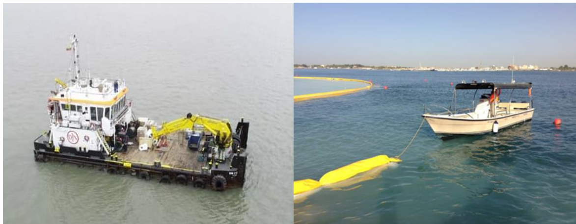
Figure 3-9: Typical vessels used for the installation, maintenance and removal of silt curtains
