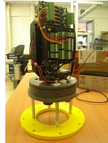
The contents of the water-tight container. The OMC-045-III logger is clearly visible.
