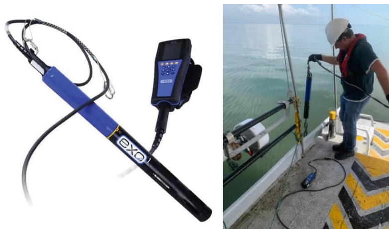
Figure 3-14: Typical mobile turbidity monitoring setup
