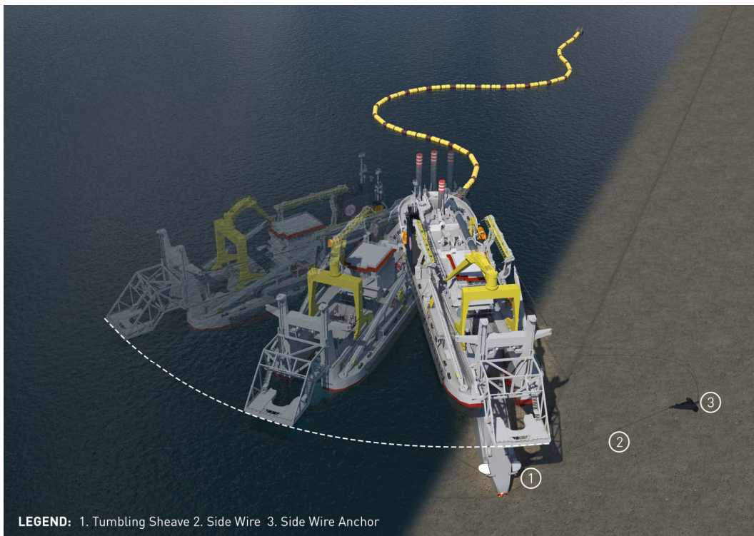
Figure 3-1: The CSD swinging left to right during dredging with help of side wire (2) and side wire anchor (3) that connect to the cutter ladder via the tumbling sheave (1)
