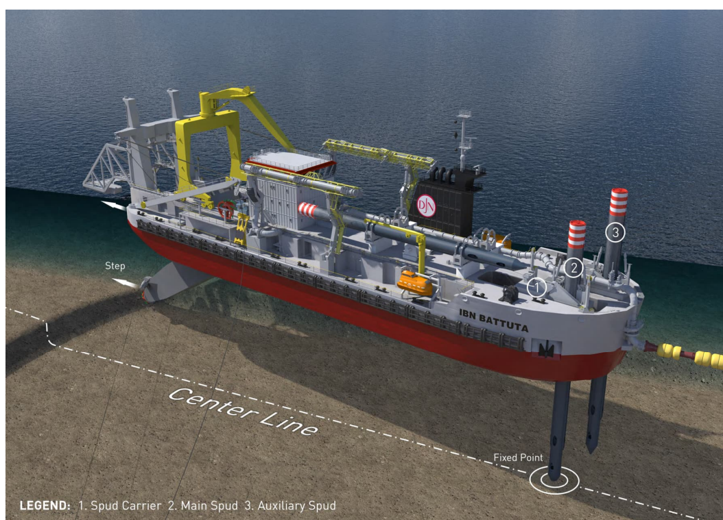
Figure 4-1: The CSD moves forward by pushing via the spud carrier (1) on the main spud (2), while the auxiliary spud (3) is used to hold the CSD in position while the main spud is repositioned
