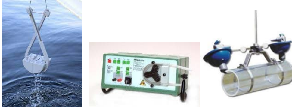
Figure 3-16: Water and sediment sampling equipment: Van Veen grab (left), peristaltic pump and Van Dorn bottle (right)
