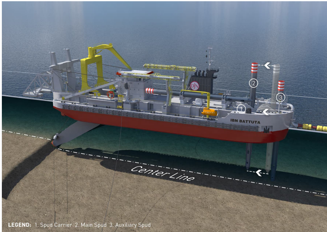
Figure 4-2: The CSD retracts the spud carrier (1) by dropping the auxiliary spud (3) and raising the main spud (2)
